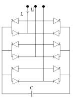
Fig.2. Three-phase scheme of STATCOM
