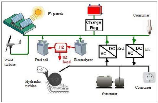
Fig.1. Scheme of an autonomous hybrid system
