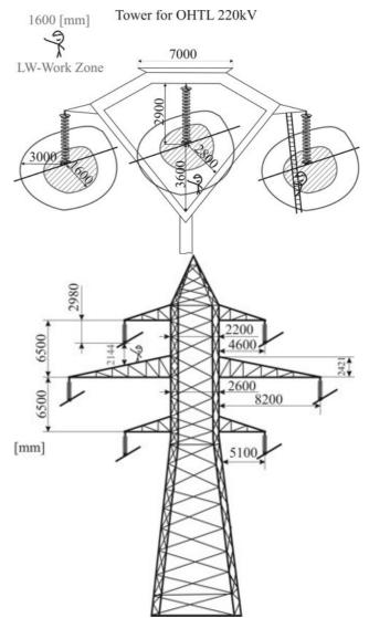
Fig.3. Clearance distances for works at 220kV OHTL
