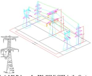
Fig.6. LW Polygon for 220-400kV OHL in the Centre for training [8]
