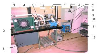
Fig.2. Subsystem wind hydro- physical model CHHE - overview: 1 - water tank; 2 - Pelton hydraulic turbine; 3 - Pump; 4 - digital manometer; 5 - Prize INVERTER OUTPUT; 6 - Remote inverter; 7 - Electric panel; 8 - Battery charging controller; 9 - Inverter; 10 - Battery; 11 - Dump load; 12 - hydro load resistors.
