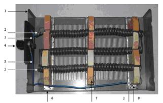
Fig.4. The load resistance: 1 - housing; 2 - clamp connection; 3 - wire connection; 4 - Connection terminals; 5 - wire resistive twisted; 6 - guide rail; 7 - ceramic pieces; 8 - fasteners.
