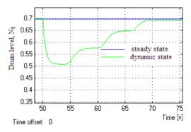
Fig. 3. Provided with system response regulator (sensitivity 150, from 6 [s])
