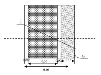
Fig. 2. Exterior wall with insulation thickness, d =0.15 m
