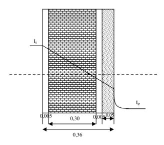
Fig. 1. Exterior wall with insulation thickness, d =0.05 m
