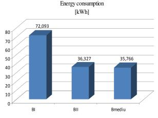
Fig. 3. Energy consumption for different thicknesses of insulation layer including the value of average consumption
