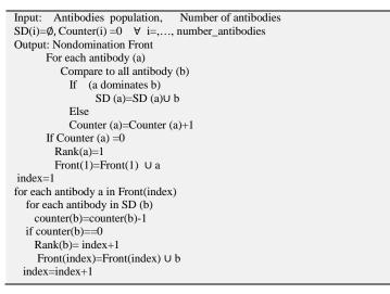
Figure 4. Algorithm Fast Non Dominated Sorting
