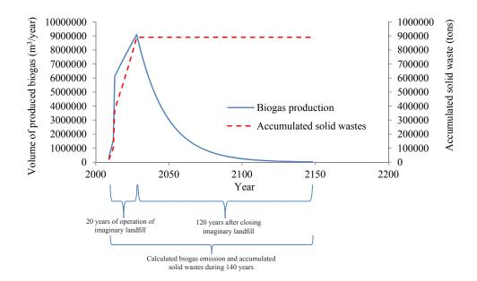
Fig. 1. Estimation of accumulated solid waste and produced biogas in the imaginary solid waste landfill of Najafabad over 140 years (2008–2148)
