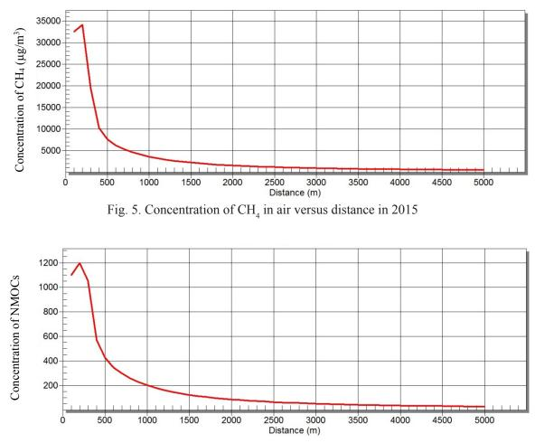
Fig. 6. Concentration of NMOCs in air versus distance in 2015
