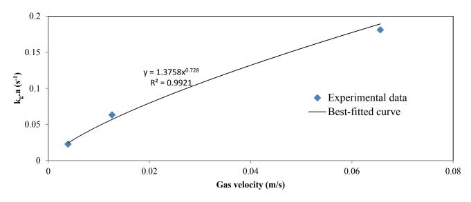
Fig.5. The variation of  $k_{o}a$  with gas velocity
