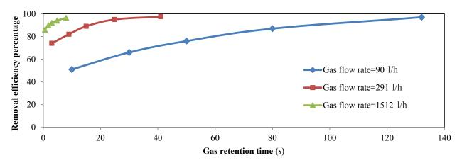
Fig.3. Formaldehyde removal efficiency versus gas retention time in the continuous BTFR for gas flow rates of 90, 291 and 1512 l/h
