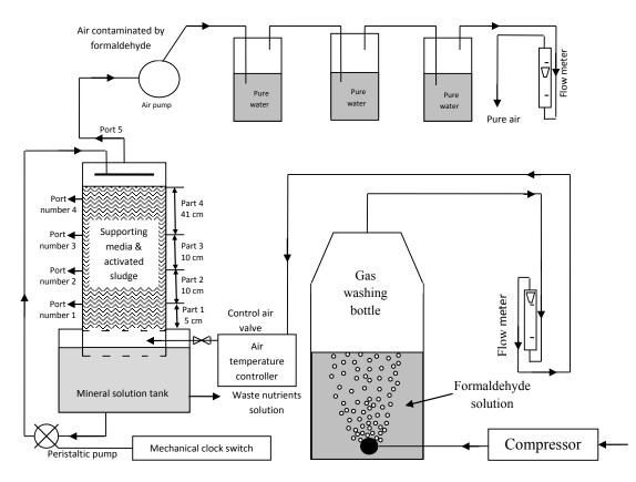
Fig.1. Schematic of the continuous BTFR and synthetic contaminated air stream (SCAS) production systems
