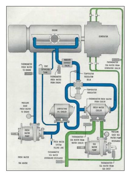
Figure 3. Fresh and salt water cooling system on a ship.
