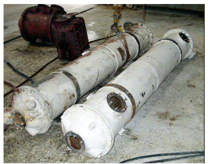
Figure 1. Seawater cooled shell and tube heat exchanger
