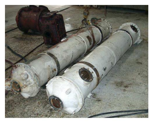
Figure 1. Seawater cooled shell and tube heat exchangers [2]
