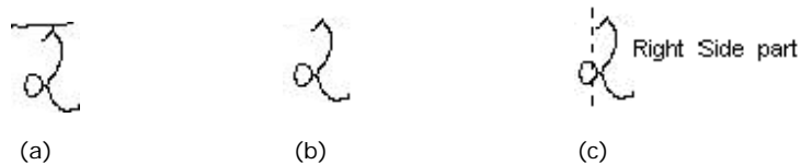
Figure 11. (a) Binarized and thinned characters image, (b) Character image after applying header line algorithm, (c) Character identified as an end-bar character
