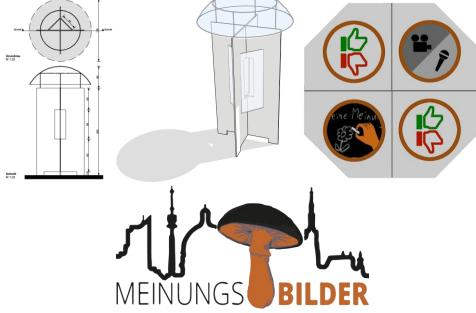
Figure 4. Interaction models: Model of the product with concrete measures for production (in this case the mushroom-shaped kiosk) (upper left), computer model to visualize the entire shape of the mushroom (upper middle), interfaces implemented in four compartments of the mushroom showing the interaction possibilities for users (upper right), the logo and corporate identity of the product (Meinungsbilder) (bottom)
