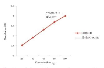
**Figure 2.** Standard curve for determination of quercitin equivalents for total flavonoid assay. Quer: Quercetin, OD: Optical Density.
