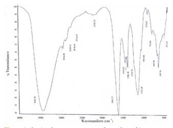
Figure 4. Showing the FT - IR spectrum of S. aculeata chitosan.
