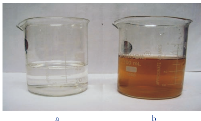
Figure 1. Photographs showing color changes after adding \text{AgNO}_3 before reaction (a) and after reaction time of 6 h (b).
