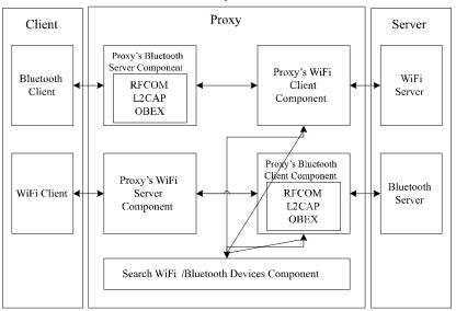
FIG. 1. HIGH-LEVEL ARCHITECTURE OF THE PROPOSED SYSTEM
