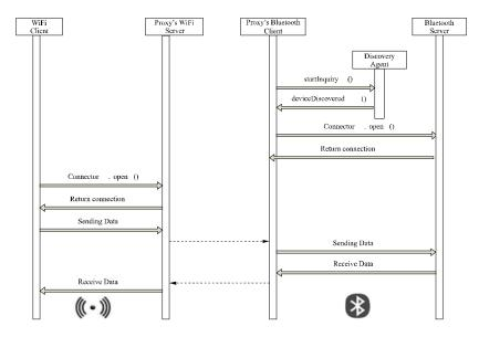
FIG. 3. INTERACTIONS BETWEEN WIFI CLIENT AND BLUETOOTH SERVER THROUGH THE PROXY
