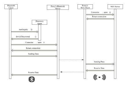
FIG. 2. INTERACTIONS BETWEEN BLUETOOTH CLIENT TO WIFI SERVER THROUGH THE PROXY
