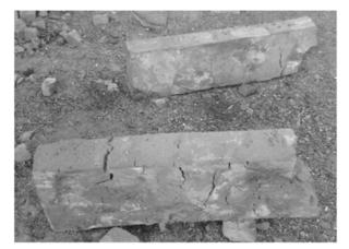
FIG. 2. THE BEAMS BAKED IN THE COMMERCIAL KILN WITHOUT APPLYING ANY TREATMENT
