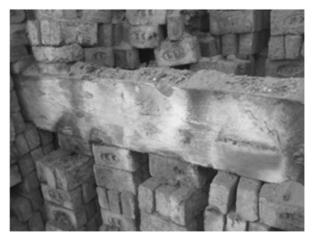
FIG. 9. BEAMS WARPED DURING THE PROCESS OF COMMERCIAL BAKING
