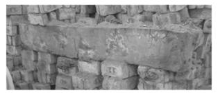
FIG. 11. CLAY BEAMS WARPED DURING BAKING IN COMMERCIAL BATHA
