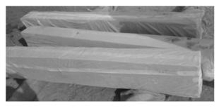
FIG. 3. BEAMS COVERED WITH PLASTIC SHEET BEFORE BAKING
