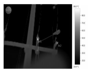
FIG. 5. THERMOGRAPH SHOWING LOSE CONNECTION AT DROP OUT FUSE ASSEMBLY OF 200KVA TRANSFORMER AT MUET, JAMSHORO
