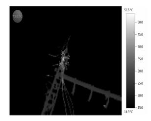
FIG. 6. THERMOGRAPH SHOWING LOSE CONNECTION AT SERVICE LINE CONNECTIONS AT MUET RESIDENTIAL SOCIETY, JAMSHORO
