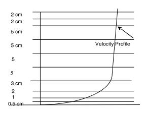
FIG. 6. MUTUAL DISTANCE ALONG THE DEPTH OF THE CHANNEL BETWEEN SUCCESSIVE POINTS OF VELOCITY MEASUREMENTS
