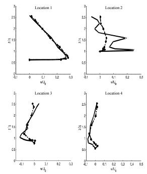
FIG. 7(B). VERTICAL VELOCITY RESULTS OVER VARIOUS POSITIONS (NON-VEGETATED CASE SHOWN BY DOTTED LINE AND SOLID LINE INDICATES VEGETATED CASE WITH Q=40 L/SEC) [w/u<sub>o</sub> represents normalized vertical velocity whereas z/Δ shows normalized depth of flow with reference to weir height (Δ)]
