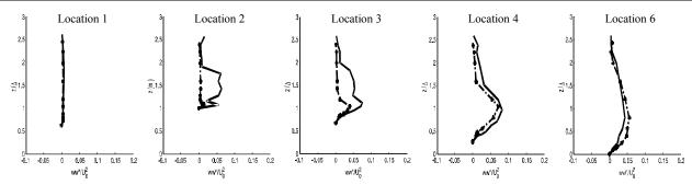
FIG. 10(B). REYNOLDS NORMAL STRESS (WW) RESULTS OVER VARIOUS POSITIONS (NON-VEGETATED CASE SHOWN BY DOTTED LINE AND SOLID LINE INDICATES VEGETATED CASE WITH Q=40 L/SEC) [ww"/u $_o$ <sup>2</sup> represents normalized Reynolds normal stresses whereas  $z/\Delta$  shows normalized depth of flow with reference to weir height ( $\Delta$ )]
