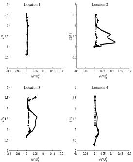
FIG. 8(C). REYNOLDS NORMAL STRESS (WW) RESULTS OVER VARIOUS POSITIONS (NON-VEGETATED CASE SHOWN BY DOTTED LINE AND SOLID LINE INDICATES VEGETATED CASE WITH Q=40 L/SEC) [ww"/u₀² represents normalized Reynolds normal stresses whereas z/Δ shows normalized depth of flow with reference to weir height (Δ)]
