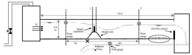
FIG. 2. A VIEW OF THE FLUME USED IN THE EXPERIMENTATION
