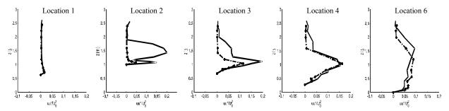
FIG. 10(A). REYNOLDS NORMAL STRESS (UU) RESULTS OVER VARIOUS POSITIONS (NON-VEGETATED CASE SHOWN BY DOTTED LINE AND SOLID LINE INDICATES VEGETATED CASE WITH Q=40 L/SEC) [uu"/ $u_o^2$  represents normalized Reynolds normal stresses whereas  $z/\Delta$  shows normalized depth of flow with reference to weir height  $(\Delta)$ ]
