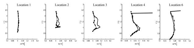
FIG. 9(B). REYNOLDS NORMAL STRESS (WW) RESULTS OVER VARIOUS POSITIONS (NON-VEGETATED CASE SHOWN BY DOTTED LINE AND SOLID LINE INDICATES VEGETATED CASE WITH Q=25 L/SEC) [ww"/ $u_o^2$  represents normalized Reynolds normal stresses whereas  $z/\Delta$  shows normalized depth of flow with reference to weir height  $(\Delta)$ ]
