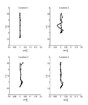
FIG. 8(A). REYNOLDS SHEAR STRESS RESULTS OVER VARIOUS POSITIONS (NON-VEGETATED CASE SHOWN BY DOTTED LINE AND SOLID LINE INDICATES VEGETATED CASE WITH Q=40 L/SEC) [uw"/u₀² represents normalized Reynolds shear stresses whereas z/Δ shows normalized depth of flow with reference to weir height (Δ)]
