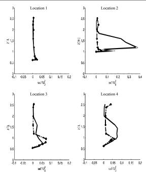
FIG. 8(B). REYNOLDS NORMAL STRESS (UU) RESULTS OVER VARIOUS POSITIONS (NON-VEGETATED CASE SHOWN BY DOTTED LINE AND SOLID LINE INDICATES VEGETATED CASE WITH Q=40 L/SEC) [uu"/u₀² represents normalized Reynolds normal stresses whereas z/Δ shows normalized depth of flow with reference to weir height (Δ)]
