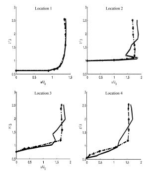
FIG. 7(A). PRIMARY VELOCITY RESULTS OVER VARIOUS POSITIONS (NON-VEGETATED CASE SHOWN BY DOTTED LINE AND SOLID LINE INDICATES VEGETATED CASE WITH Q=40 L/SEC) [u/u<sub>o</sub> represents normalized stream-wise velocity whereas z/\(\Delta\) shows normalized depth of flow with reference to weir height (\Delta\)]
