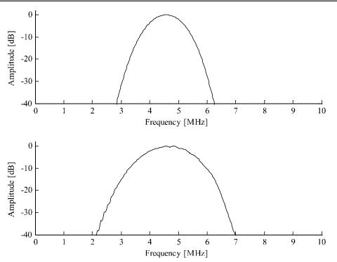
FIG. 7. THE AMPLITUDE SPECTRA OF EXTRACTED SECOND HARMONIC CHIRP SIGNALS OBTAINED UNDER CHIRP EXCITATION WITH -6dB FRACTIONAL BANDWIDTH OF 44.2% (TOP) AND 66.7% (BOTTOM) RESPECTIVELY
