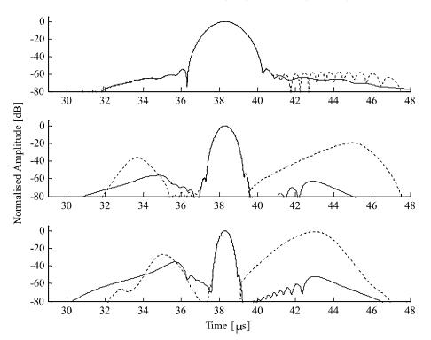
FIG. 8. THE COMPARISON OF UNFILTERED (DASHED LINE) AND FRFT PRE-FILTERED (SOLID LINE) HARMONIC MATCHED FILTERED COMPRESSED SIGNALS OBTAINED USING CHIRP EXCITATION WITH -6dB FRACTIONAL BANDWIDTH OF 22.6% (TOP), 44.2% (MIDDLE) AND 66.7% (BOTTOM) RESPECTIVELY
