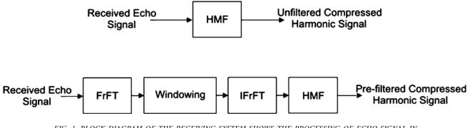
FIG. 1. BLOCK DIAGRAM OF THE RECEIVING SYSTEM SHOWS THE PROCESSING OF ECHO SIGNAL IN CONVENTIONAL (TOP) AND PROPOSED (BOTTOM) METHODS
