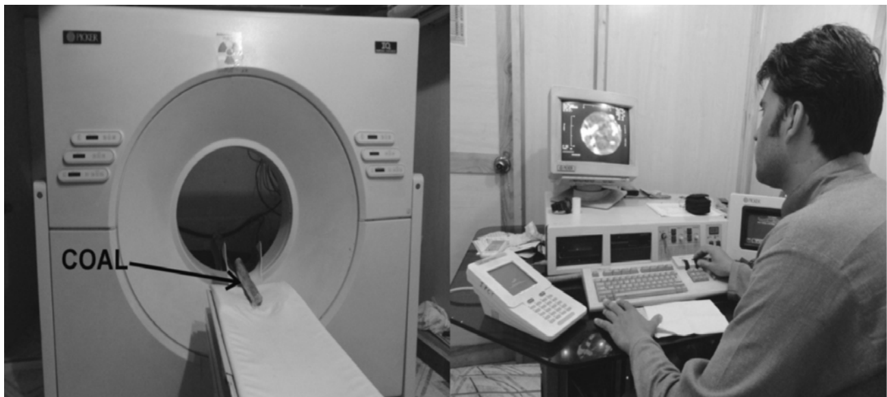
FIG. 2.SHOWING X-RAY COMPUTED TOMOGRAPHIC SCANNING MACHINE.
