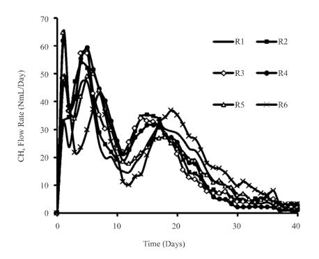
(b) METHANE FLOW RATE; (R1= 10:90; R2= 20:80; R3= 30:70; R4= 40:60; R5= 50:50; R6= 60:40) FIG. 2. METHANE PRODUCTION AT DIFFERENT CANOLA STRAW TO BUFFALO DUNG RATIO
