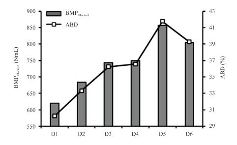
FIG. 5. COMPARISON OF BMP AND ABD AT DIFFERENT ALKALINE DOZES; (D1=0.2; D2=0.3; D3=0.4; D4=0.5; D5=0.6; D6=0.7 gNaHCO/gVS)
