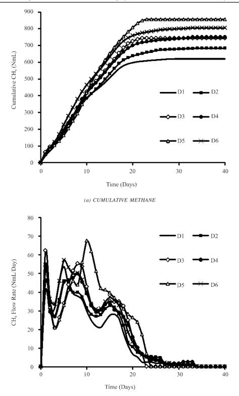
(b) METHANE FLOW RATE; (D1=0.2; D2=0.3; D3=0.4; D4=0.5; D5=0.6; D6=0.7 gNaHCO<sub>3</sub>/gVS)
