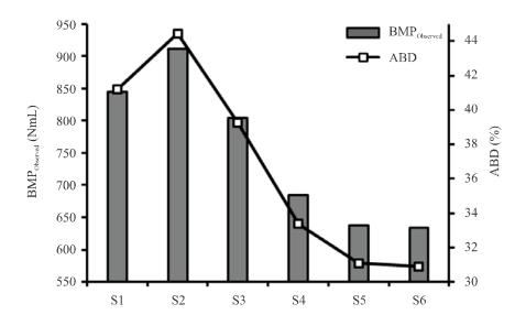
FIG. 7 COMPARISON OF BMP AND ABD AT DIFFERENT CANOLA STRAW PARTICLE SIZES; (S1<1; S2=2; S3=4; S4=6; S5=8; S6=10mm)
