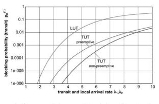
FIG. 13. LUT VERSUS TUT BLOCKING OF LOSS TRAFFIC VERSUS BOTH ARRIVAL RATES  $\lambda_2$  AND  $\lambda_2$
