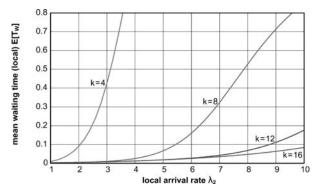
FIG. 11. LUT MEAN WAITING TIME LOCAL TRAFFIC WITH WITH VARYING THRESHOLDS OF 4.8.12.16 WITH TRANSIT LOAD = 10, W=16, S=10
