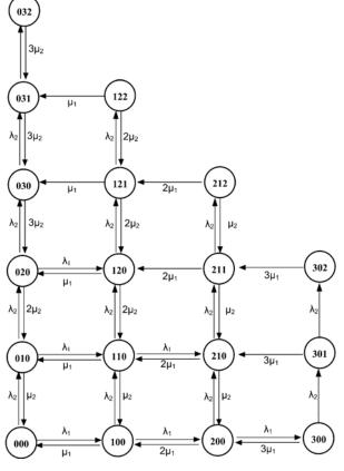
FIG. 5. STATE DIAGRAM OF A AN EXAMPLE M/M/N/S MIXED LOSS DELAY SYSTEM WITH NO THRESHOLDS WHERE N=3, S=5
