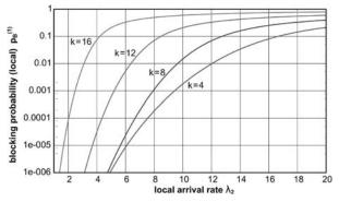
FIG. 9. LUT BLOCKING PROBABILITY OF LOCAL TRAFFIC WITH VARYING THRESHOLDS OF 4.8.12.16 WITH TRANSIT LOAD = 10, W=16, S=10
