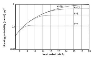
FIG. 10. LUT BLOCKING PROBABILITY OF LOCAL TRAFFIC WITH VARYING THRESHOLDS OF 4.8.12.16 WITH TRANSIT LOAD = 10, W=16, S=10
