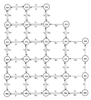
FIG. 6. STATE DIAGRAM OF AN EXAMPLE M/M/N/S MIXED LOSS DEALY SYSTEM WITH LOCAL USAGE BASED THRESHOLD OLD (K) WHERE N=4, S=7, AND K=2
