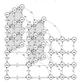
FIG. 8. STATE DIAGRAM OF AN EXAMPLE M/M/N/S MIXED LOSS DEALY SYSTEM WITH TOTAL USAGE BASED THRESHOLD OLD (K) WITHOUT PREEMPTION OF LOCAL TRAFFIC WHERE N=4, S=7, AND K=2
