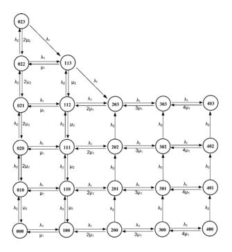
FIG. 7. STATE DIAGRAM OF AN EXAMPLE M/M/N/S MIXED LOSS DEALY SYSTEM WITH TOTAL USAGE BASED THRESHOLD OLD (K) AND PREEMPTION OF LOCAL TRAFFIC WHERE N=4, S=7, AND K=3
