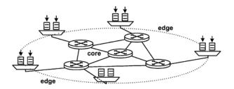
(a) SEPARATION OF EDGE AND CORE PARTS
