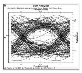
FIG. 14. RAMAN AMPLIFIER PERFORMANCE AT 170KM
