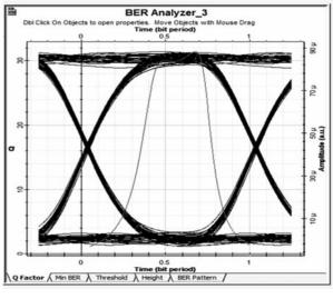
FIG. 12. RAMAN AMPLIFIER PERFORMANCE AT 120KM
