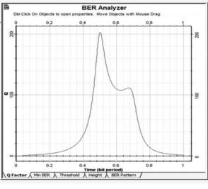
FIG. 8. Q-FACTOR OF RAMAN AMPLIFIER AT 60KM
