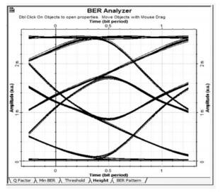
FIG. 9. EDFA EYE DIAGRAM BY CONSIDERING SMF AND DCF AT 100KM
