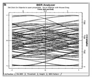
FIG. 11. EDFA EYE DIAGRAM WITH SMF AND DCF CONSIDERATION AT 120KM
