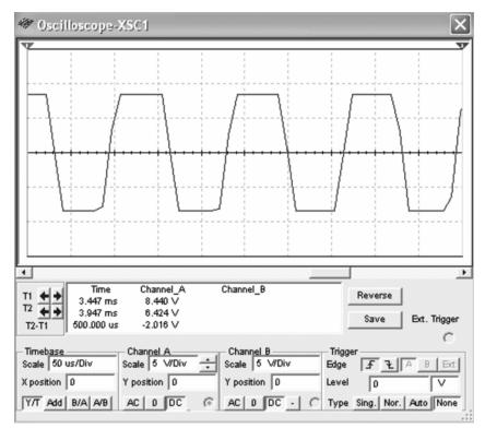
FIG. 5. PWM SIGNAL WHEN VS=10V<sub>P-PK</sub>
