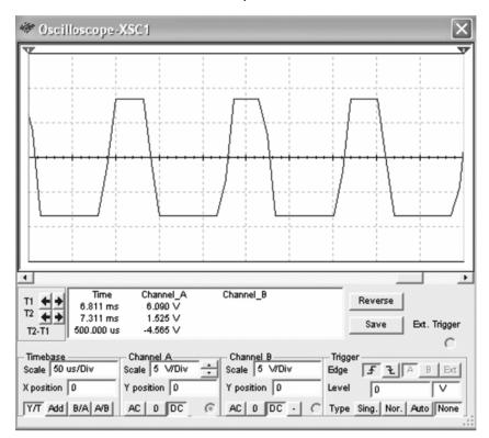
FIG. 6. PWM SIGNAL WHEN VS=15V<sub>P-PK</sub>
