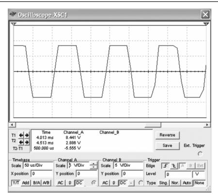
FIG. 4. PWM SIGNAL WHEN VS=5V<sub>P-PK</sub>
