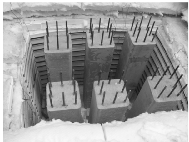
FIG. 2. ARRANGEMENT OF POST-HEATED SQUARE REINFORCED CONCRETE COLUMNS IN FURNACE
