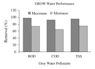
FIG. 6. GROW SYSTEM PERFORMANCE WITH MAXIMUM AND MINIMUM REMOVAL (%)
