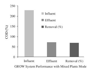
FIG. 3. INFLUENT AND EFFLUENT QUALITY IN TERMS OF COD REMOVAL PERCENTAGE
