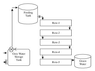
FIG.1. SCHAMATIC DIAGRAM OF THE GROW SYSTEM
