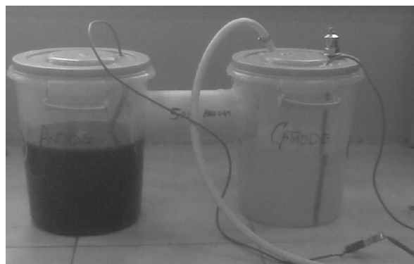
FIG. 1. CAMERA IMAGE OF PROTOTYPE MICROBIAL FUEL CELL
