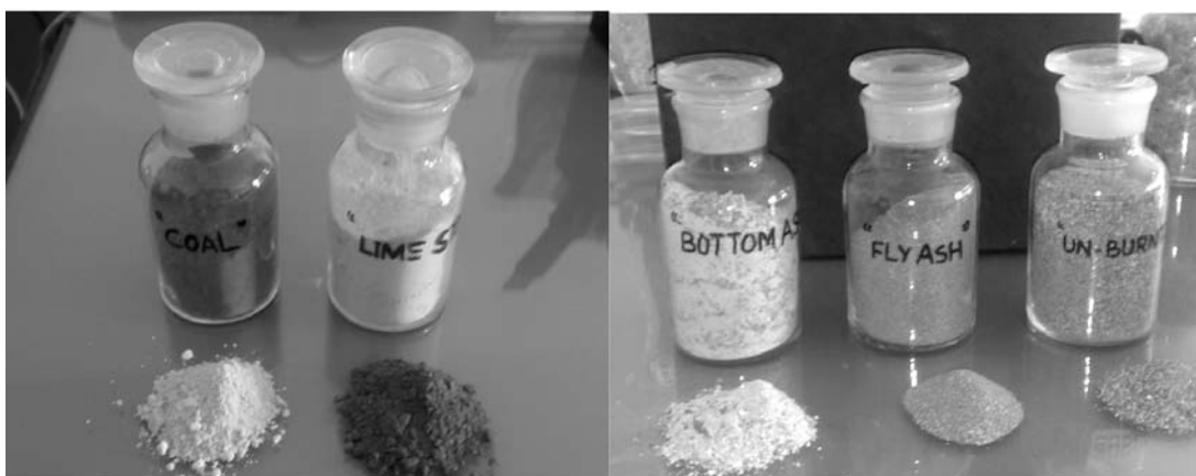
FIG 1. SAMPLES OF COAL, LIMESTONE, BOTTOM ASH, FLY ASH AND UN-BURNT MATERIALS
