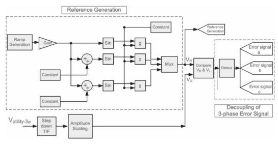
FIG. 4. BLOCK DIAGRAM REPRESENTATION TO GENERATE ERROR SIGNAL
