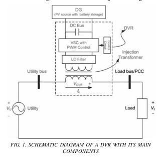
load current needs not be 90 and can theoretically have any value. A DG as an energy source connected to DClink of DVR is shown in Fig. 1.
