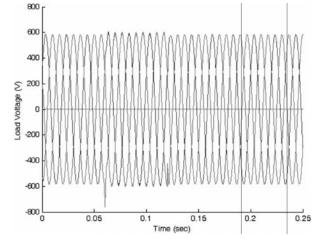
FIG. 17. LOAD VOLTAGE AFTER COMPENSATING AN UNBALANCED SWELL IN 3-PHASE UTILITY VOLTAGE
