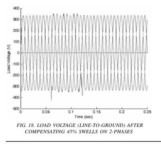
generated by DVR according to the developed control strategy to regulate load voltage. The load voltage is kept near to its nominal value as evident by solid line in the plot.
