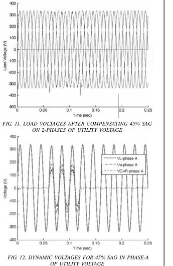
The dynamic voltages, active powers and reactive powers for load, utility and DVR are plotted for only Phase-A of 3phase system to show sag mitigation by the DVR for the proposed control strategy. However, plots of dynamic voltages, active powers and reactive powers for the other 2-phases can be obtained on the similar analogy.
