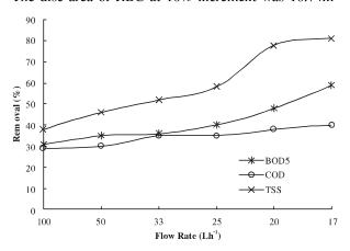
FIG. 2. REMOVAL PERCENTAGE OF BOD<sub>5</sub>, COD, AND TSS AT SIX FLOW RATES
