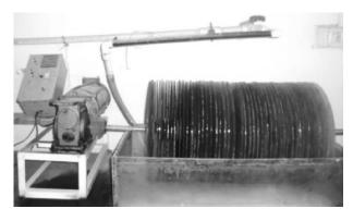
FIG.2. ROTATING BIOLOGICAL CONTACTOR
