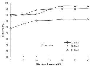
FIG. 6. REMOVAL PERCENT OF TSS AT THREE FLOW RATES
