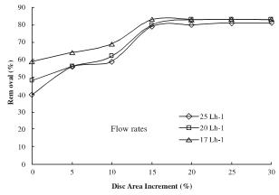
FIG. 4. REMOVAL PERCENT OF BOD5 AT THREE FLOW RATES
