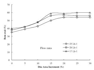
FIG. 5. REMOVAL PERCENT OF COD AT THREE FLOW RATES
