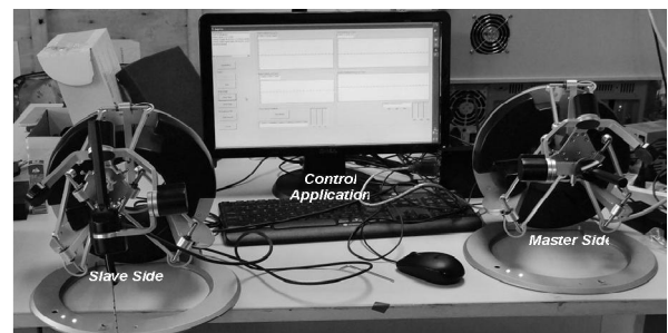
FIG. 2. PROPOSED MASTER/SLAVE SYSTEM
