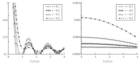
FIG. 2. PLOT OF THE VELOCITY FIELD AND THE SHEAR STRESSF ROM EQUATIONS (18) AND (24), FOR M,P,U,A, AND T WITH VALUES 1.52, 2.413,1, 2, AND 2 S RESPECTIVELY FOR VARIOUS VALUES OF N
