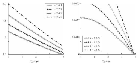
FIG. 1. PLOT OF THE VELOCITY FIELD AND THE SHEAR STRESSF ROM EQUATIONS (18) AND (24), FOR M,N,U,A, AND  $\Omega$  WITH VALUES 1.52, 0.63,2, 2, AND 2 FOR VARIOUS VALUES OF T
