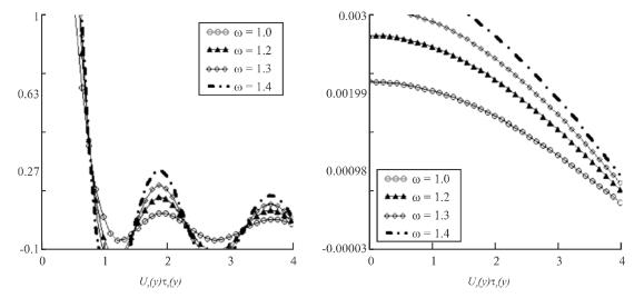
FIG. 4. PLOT OF THE VELOCITY FIELD AND THE SHEAR STRESS FROM EQUATIONS(18) AND (24), FOR M,N,U,A, AND WITH VALUES 1.52, 0.63,1, 2, AND 2 RESPECTIVELY FOR VARIOUS VALUES OF  $\Omega$
