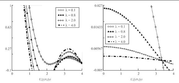
FIG. 3. PLOT OF THE VELOCITY FIELD AND THE SHEAR STRESS FROM EQUATIONS(18) AND (24), FOR  $M,N,U,\Omega$ , AND WITH VALUES 1.52, 0.63,1,2, AND 2 RESPECTIVELY FORVARIOUS VALUES OF  $\Lambda$
