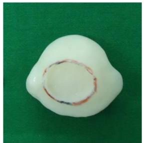
Fig. 6: Trough created to place iris replica
