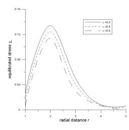
**Fig.** 7 – Variation of equilibrated stress  $\chi_r$  w.r.t. radial r.
