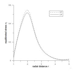
Fig. 2 – Variation of equilibrated stress  $\sigma_r$  w.r.t. radial distance r.
