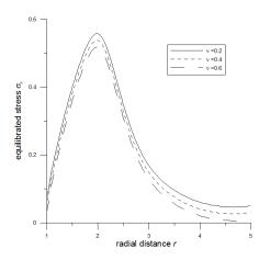
**Fig.** 6 – Variation of equilibrated stress  $\sigma_r$  w.r.t. radial distance r.
