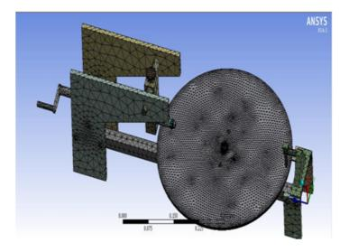
Fig. 4 – Meshing of the designed part (Ansys workbench).
