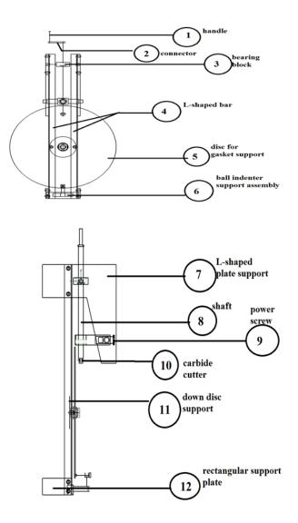
Fig. 3 – Schematic model of gasket cutting machine.
