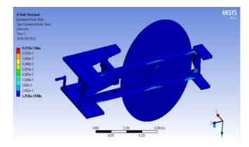
Fig. 8 – Von-Mises strain analysis of the designed model (Ansys workbench).
