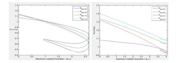
Fig. 7 – PV curves before and after placement of UPFC's (Voltage Dependant Load).
