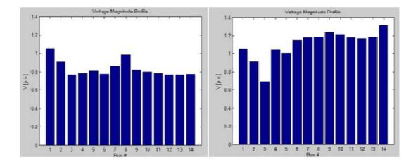
**Fig.** 10 – Voltage magnitude profile before and after placement of UPFC's (Exponential Recovery Load).
