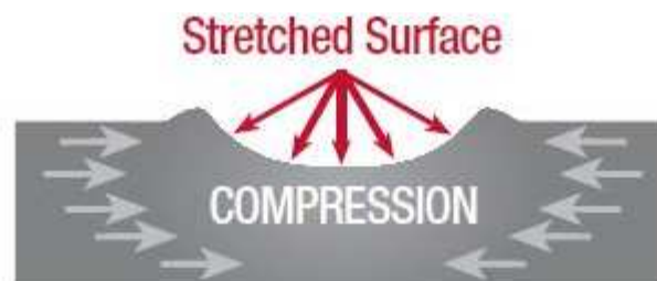
Figure 2: Compression Resists Fatigue Cracking
