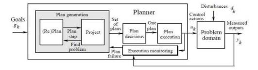
Figure 5: Closed Loop Planning Control System
