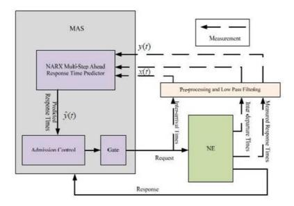
Figure 15: Mutli-Step Ahead Response Time Predictor
