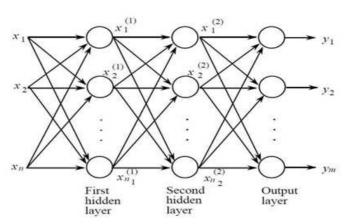
Figure 2: A 3-Layer Multi Perceptron Model
