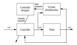
Figure 6: Indirect Adaptive Control
