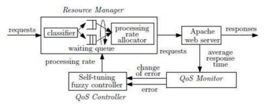
Figure 11: System Architecture of Apache Server STFC
