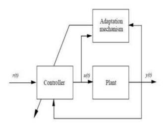
Figure 7: Direct Adaptive Control
