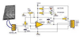
**Figure 2: The Rain Sensor Module**
