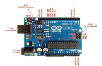
Figure 3: Arduino UNO Based on ATMega-328 Microcontroller
