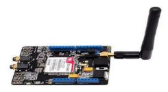
Figure 4: GSM MODEM- SIM900
