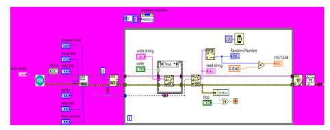
Figure 6: Block Diagram of LabVIEW based Rain Fall Detector with Arduino
