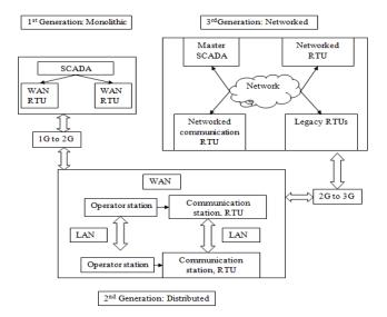
**Figure 2: SCADA Systems Evolution**
