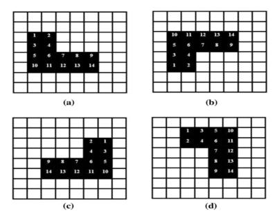
Figure 2: (a) Original 8 \* 8 Image and Its Resulting Output Images after Applying in (b) The Vertical Flip, (c) The Horizontal Flip, and in (d) the Coordinate Swap Operations, Respectively
