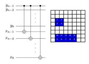
Figure 4: The Control on the Yn\_1 Qubit in the Circuit on the Left Divides an Entire Image Into It's Upper and Lower Halves. Using This Control, the Circuit on the left shows how the Flip Operation Can Be Confined to the Lower Half of an Image. The Figure to its Right Shows the Effect of Such a Transformation on the 8 \* 8 Binary Image in Figure 2(A)
