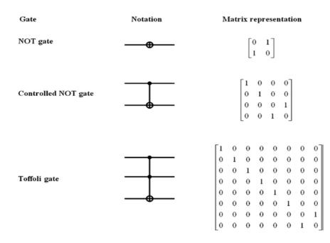
Figure 1: Representing Various Gates Used in Quantum Computation
