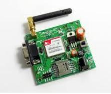
Figure 3.6.1: GSM Modem
