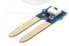
Figure 3.4.1: Soil Moisture Sensor
