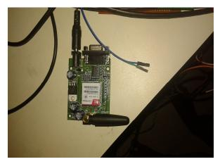
Figure 6.4: GSM Modem
