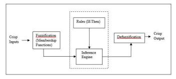
Figure 2 Block diagram of Fuzzy Logic Controller
