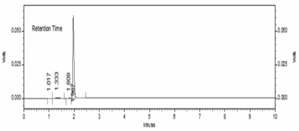
Fig. 2: A typical HPLC chromatogram of 5-Fluorouracil (5-FU)
