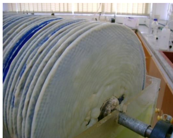
Figure 9. Biofilm developed on rotating discs of the NRBC system
