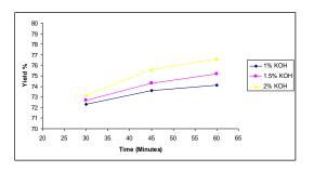
**Figure 5** Effect of molar ratio 4.5:1 for biodiesel from mixture of 25% karanja and 75% linseed oil
