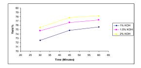
Figure 2 Effect of molar ratio 6:1 for biodiesel from mixture of 50% karanja and 50% Linseed oil
