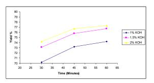
**Figure 1.** Effect of molar ratio 4.5:1 for biodiesel from mixture of 50% karanja and 50% linseed oil
