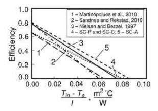
Figure 9 - Thermal efficiency of the different SCs.
