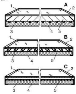
*Figure 2* – Schematic diagrams of the studied solar collectors structure: A – SC with aluminum absorber (SC-A), B – SC with copper tubes (SC-C), C – polymeric SC (SC-P). 1 – transparent cover, 2 – frame, 3 – thermal insulation; 4 – bottom; 5 – absorber
