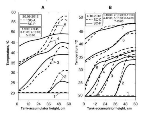
*Figure 8* – Comparative data for the water temperature distribution in the tank-accumulator for the SC-A and SC-P (A), and for the SC-C and SC-P (B).
