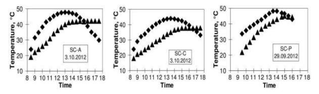
*Figure 6* – Water temperature at the exit of SC (♦) and the average temperature in the tank-accumulator (▲) for SC-A, SC-C, and SC-P.
