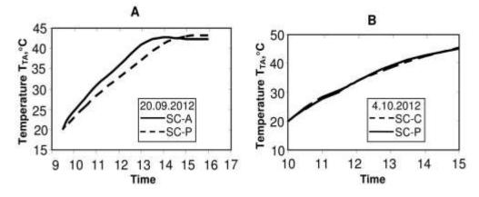
*Figure* 7 – Comparative data for the average water temperature in the tank-accumulator for the SC-A and SC-P (A), and for the SC-C and SC-P (B).
