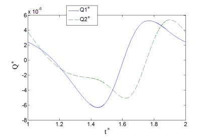
Figure 6 - Heat transfer  $Q^*$  throughout the cycle in each chamber. Heat transfer from the walls to the helium is positive, so chamber 1 (expansion space) has a net cooling effect on the chamber wall, while chamber 2 (compression space) has a net heating effect on the chamber wall.
