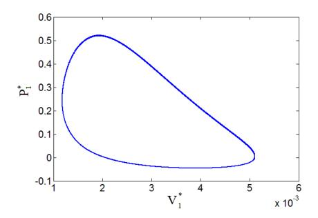
Figure 2 - Pressure-volume diagram for chamber 1 over a cycle.
