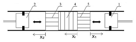
Figure 1 - Alpha Stirling refrigerator 1 - the expander, 2 - the compressor, 3 - the warm heat exchanger, 4 - the regenerator, 5 - the cold heat exchanger. The arrows point in the positive direction for each coordinate.
