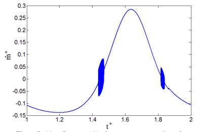
Figure 5 - Mass flow rate m<sup>\*</sup> in the regenerator over the cycle. The slight mass flow rate fluctuation around 0 is numerical due to the change of sign of the velocity.
