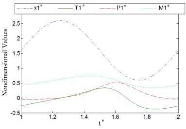
Figure 3 - Helium temperature  $T_1^*$  (solid -), pressure  $P_1^*$  (dashed - - ) and mass  $M_1^*$  (dotted ...) in chamber 1 over a cycle. This also shows the chamber 1 piston motion  $x_1^*$  (dash-dot -.).
