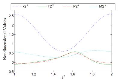
Figure 4 - Helium temperature  $T_2^*$  (solid -), pressure  $P_2^*$  (dashed - -) and mass  $M_2^*$  (dotted ..) in chamber 2 over a cycle. This also shows the chamber 2 piston motion  $x_2^*$  (dash-dot -.).
